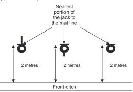
B.3.2 Position of the jack alongside a 2-metre measuring device
